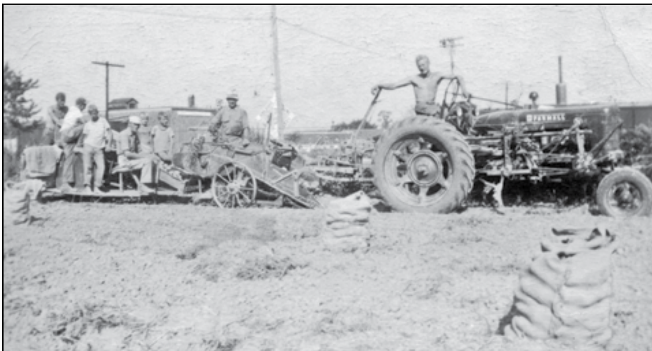
Chet helped his father plant and harvest potatoes as part of his contribution to the family farm. In the photo to the left, Chet drives the tractor that pulls the potato digger, a machine that conveys potatoes into bins so they can be placed into burlap bags.
